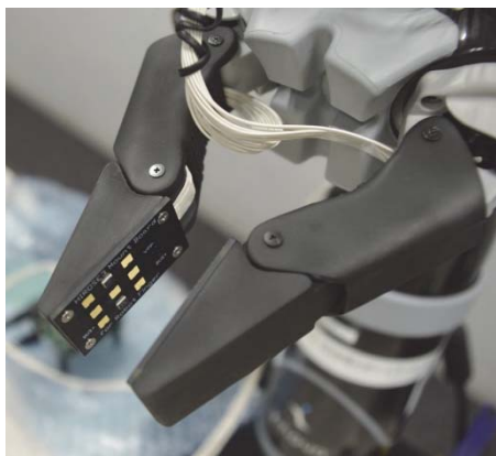
Fig. 1 Bus-network integrated tactile sensor on robot fingers
